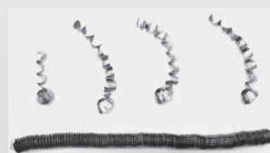
Chips by SM chipbreaker (SUS304)
